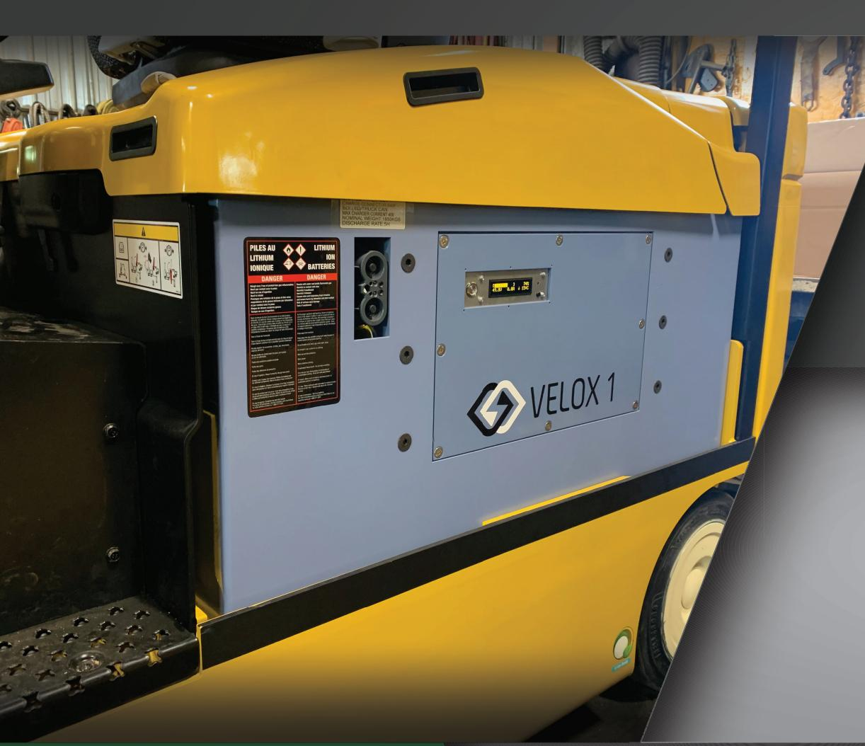
Charge your batteries during coffee and lunch breaks with a smart charger designed for Li-ion fast charging. This method can supply enough energy capacity required for work up to three shifts, 7 days a week.
